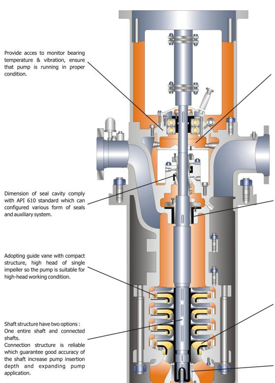
Adopting slide bearing structure, using of thin oil lubrication.
