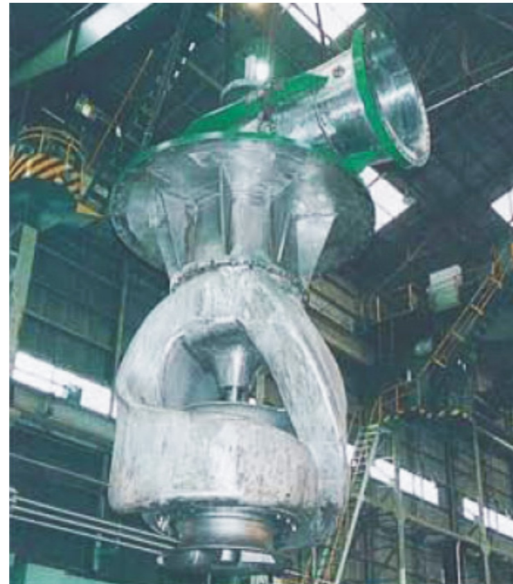
CDKTV Hot Well Pump , for 110 MW Geothermal Power Plant Chevron Texaco Energy Indonesia (Derajat II) Indonesia.
